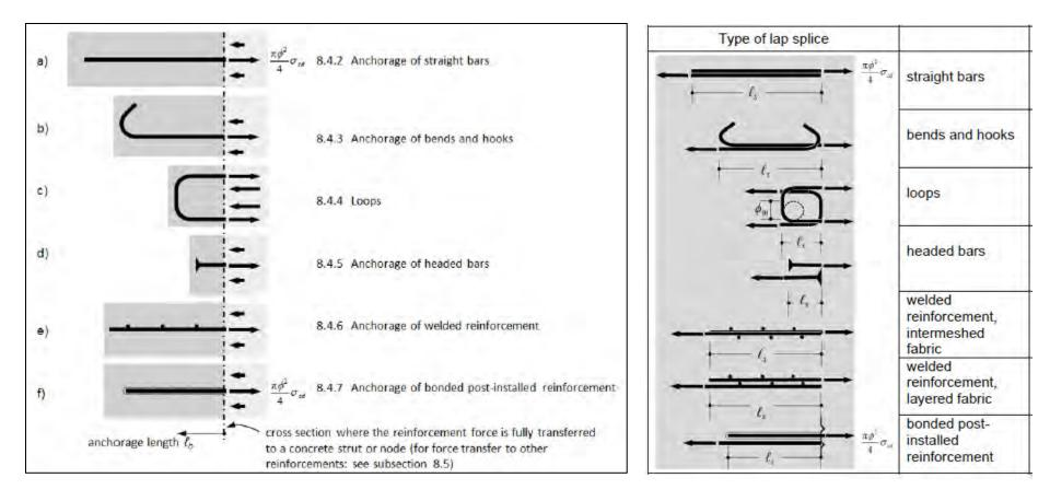
• 11.4 – Anchorage of reinforcing steel bars:
