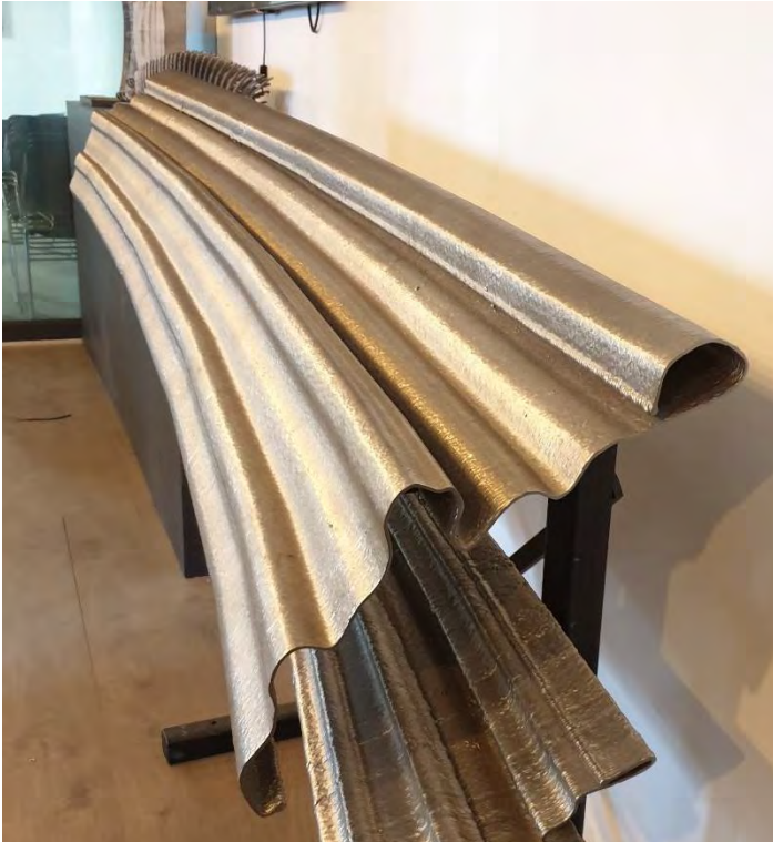
METAL CURVED PANELS, MX3D AMSTERDAM
